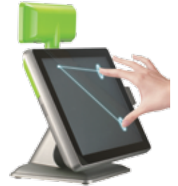
Projected Capacitive technology (PCT) & multi-touch function
